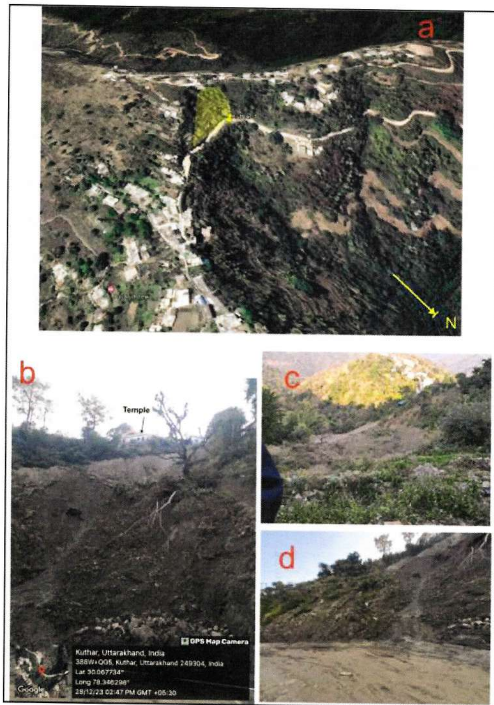
Figure 7 (A) Satellite view of Kuthar village. The yellow highlighted portion is of landslide occurred on 17 August 2023. (b) landslide view and location of temple just above the crown (c) view of landslide from the top of the crown (d) the landslide site sloping towards north hence not received sunrays for longer hours and slope material is still wet with water on road even during winter
