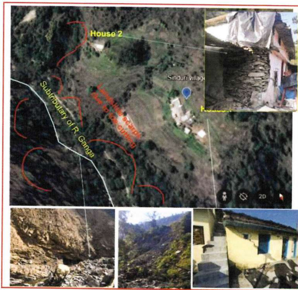
Figure 8 Field conditions and condition of houses in Veerkaatli tok of Sinduri village (Red arcuate portions denote landslide scarps developed in the monsoon of 2023)
