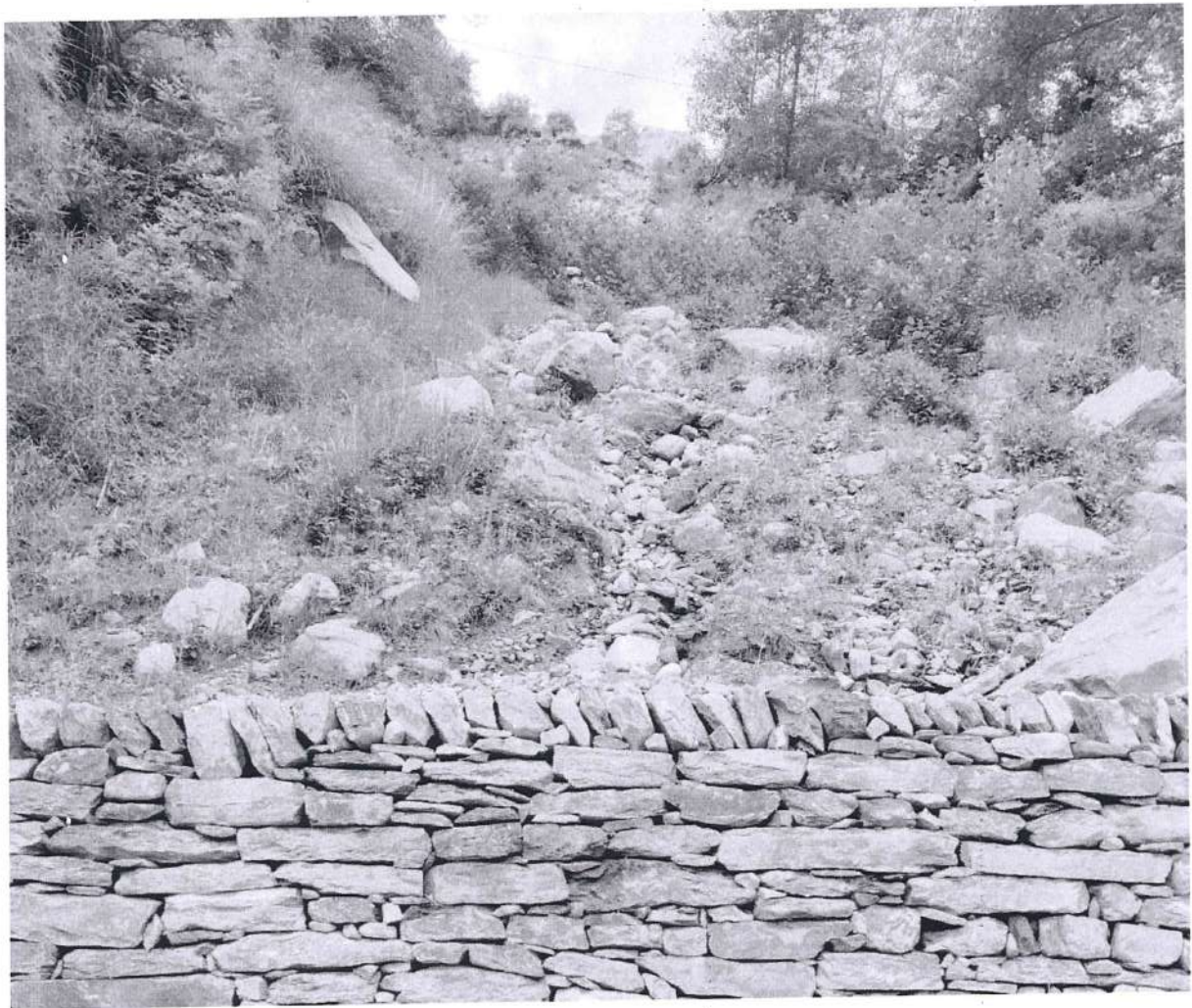
Figure 3: Field photograph showing a slope failure in the Garbha Dhar area, near Jipti village, Dharchula tehsil, Pithoragarh district. The failed slope consists of heterogeneous material, including slope wash deposits, colluvium, and large boulders. The exposed lithology primarily comprises augen gneiss, micaceous gneiss, and garnetiferous schist, reflecting the geological complexity and slope instability characteristic of the region.
