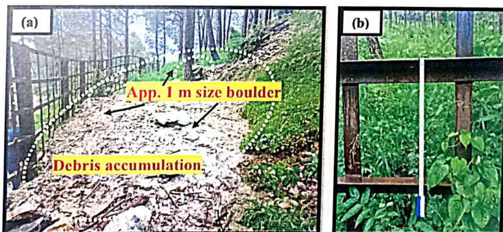
Figure 6: (a) Figure depicting the debris accumulation zone near barricade at elevation of about 1230 m and (b) size of opening of Barricade (app. 2x2 ft.)
