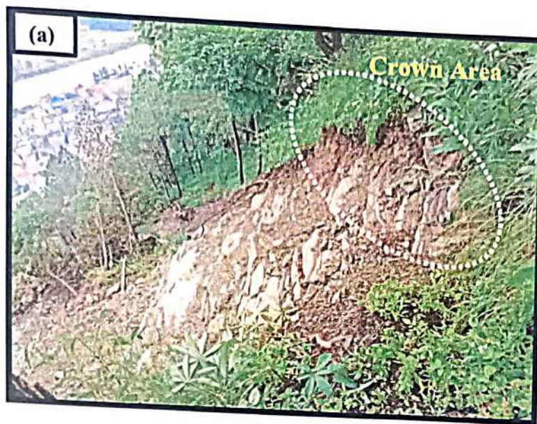
Figure 4: exhibiting middle portion of upper section where quartzite are exposed (Fig. 4a) and crushed & shattered phyllitic quartzite present at left portion (Fig. 4b) of landslide crown with hanging overburden (Fig. 4c)
