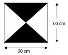
Pre-pointing Marker should be placed on firm and flat ground and should have adequate mechanism to hold it firmly to its positions during entire data acquisition period. Pre-pointing markers should be able to retain its shape and pattern even during heavy rain.
