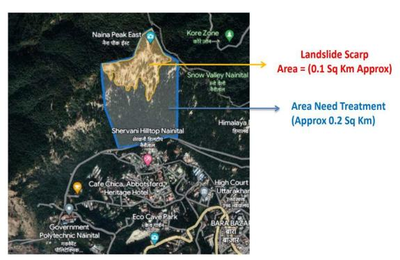
Approximate total area of 0.3 Sq. Km (0.1 sq. km of landslide scarp & 0.2 sq. Km) needs treatment for landslide.
